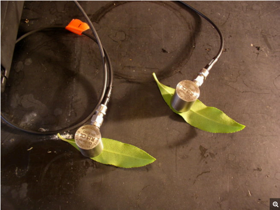
Acoustic sensors measuring hydraulic emissions from plant leaves in a Duke University laboratory.
